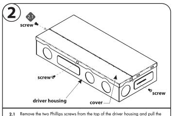
cover off to expose the driver wires.
